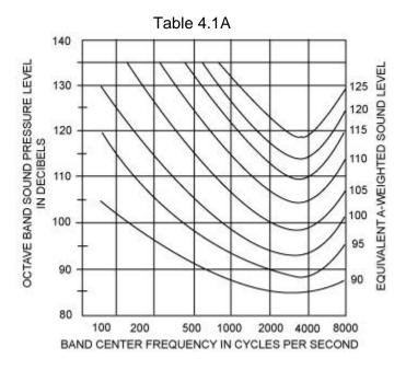
Octave band sound pressure levels may be converted to the equivalent A-weighted sound level by plotting them on this graph and noting the A-weighted sound level
